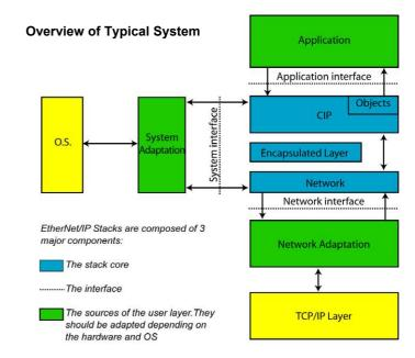
When used in scanner mode, the stack allows EtherNet/IP master features to be implemented into controller devices including PLC modules, interface cards, IPC, and robot controllers. When adapter mode is used, the stack enables EtherNet/IP slave devices such as, but not limited, to I/O modules, robots, instruments, regulators
