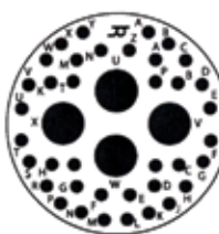
25-42 - 25-42* 38 #20, 4 #8 Coax I, Coax
