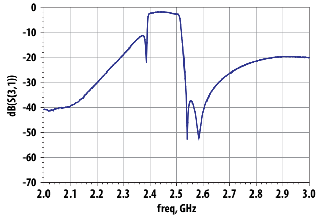
Figure 4. RX Path 2 – 3 GHz Frequency Response
