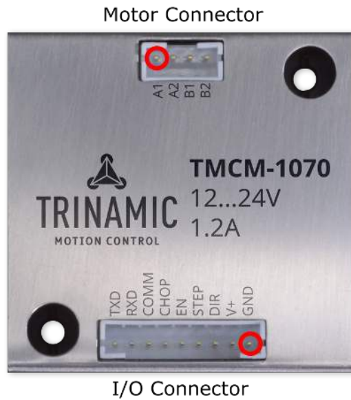
Figure 7: TMCM-1070 connectors (pin 1 highlighted in red)
