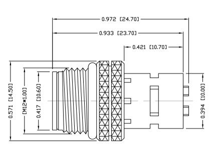
NΠΤF: MATERIAL HOUSING: PBT UL94V-0, BLACK CONTACT: BRASS NUT: BRASS □-RING: EPDM, BLACK SHELL: BRASS FINISH CONTACT: GOLD PLATED □VER 504" NICKEL NUT: NICKEL PLATED SHELL: BRIGHT TIN PLATED ELECTRICAL RATED CURRENT: 4A RATED VOLTAGE: 60V INSULATION RESISTANCE: 100 MOhms MIN. CONTACT RESISTANCE: 10 mOhms MAX. IP67 WATER PROOF: **ENVIRONMENT** -40°C TD +85°C **OPERATION TEMPERATURE:** MAX WIRE AWG: 22
