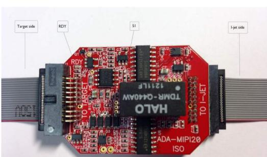
The adapter is automatically recognized by the C-SPY, and the adapter powers up and the green RDY LED is turned on.
