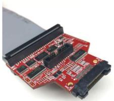
The mating connector for Mictor-38 on target board is AMP/Tyco 5767054-1.
