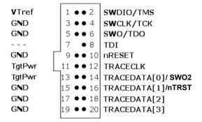
The mating connector for a target board has the part number SHF-110-01-L-D.
