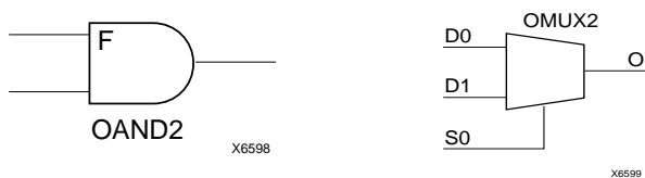
Figure 20: AND & MUX Symbols in XC4000X IOB
