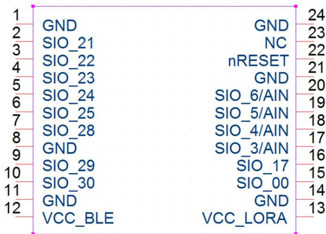
Figure 2: RM186/RM191 module pin-out (top view)
