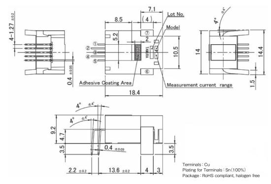
Note1) The tolerances of dimensions without any mention are  $\pm\,0.1\,\text{mm}.$
