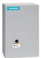
Non-reversing NEMA contactor, Size 4, Three phase full voltage, Contactor amp rating 135A, 3 wire (NO aux included), 110-120/220-240VAC 60Hz coil, Non-combination type, Enclosure NEMA type 1, Indoor general purpose use, Standard width enclosure
