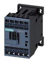
power contactor, AC-3e/AC-3, 9 A, 4 kW / 400 V, 3-pole, 12 V DC, auxiliary contacts: 1 NO, spring-loaded terminal, size: S00  $\,$
