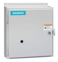
Electrically held lighting contactor, Contactor amp rating 20A, 0 N.C. / 4 N.O. Poles, 480VAC 60HZ coil, Non-combination type, (no disconnect device), Enclosure NEMA type 12, Dust/drip proof for indoors
