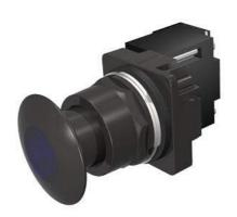
30mm BlackMax, Epoxy Coated Corrosion Resistant Complete Metal Unit Illuminated Push-Pull Operator Transformer type, 600V AC LED Lamp Mushroom Head Cap Small 1 3/4" (44.5 mm) Metal, Black with Blue Lens 3 Position Pull-Momentary/Push-Maintained UL Listed, CSA Certified NEMA 1,3,3R,4,4X,12,13 & Automotive Standards
