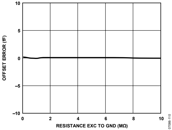
Figure 10. Capacitance Input Offset Error vs. Resistance EXC to GND, V_{DD} = 3.3\text{ V} , CIN Pin Open Circuit
