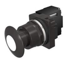
30mm BlackMax, Epoxy Coated Corrosion Resistant Complete Metal Unit Illuminated Push-Pull Operator Transformer type, 600V AC Incandescent Lamp Mushroom Head Cap Small 1 3/4" (44.5 mm) Metal, Black with White Lens 3 Position Pull-Momentary/Push-Maintained UL Listed, CSA Certified NEMA 1,3,3R,4,4X,12,13 & Automotive Standards
