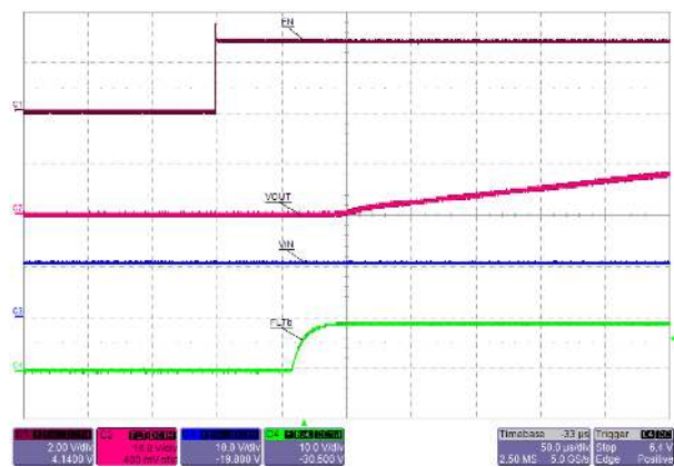
Figure 7-34. EN Turn ON Delay : EN ↑ to Output Ramp ↑
