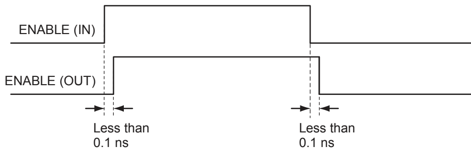
Figure 8-15 • Timing Diagram (option 1: bypasses skew circuit)
