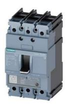
circuit breaker 3VA5 UL frame 125 breaking capacity class H 65kA @ 480 V 3-pole, line protection TM230, FTAM, In=15A overload protection Ir=15A fixed short-circuit protection Ii=10...20 x In UL489 SB (naval), 50 deg. cel. cable connection on both sides
