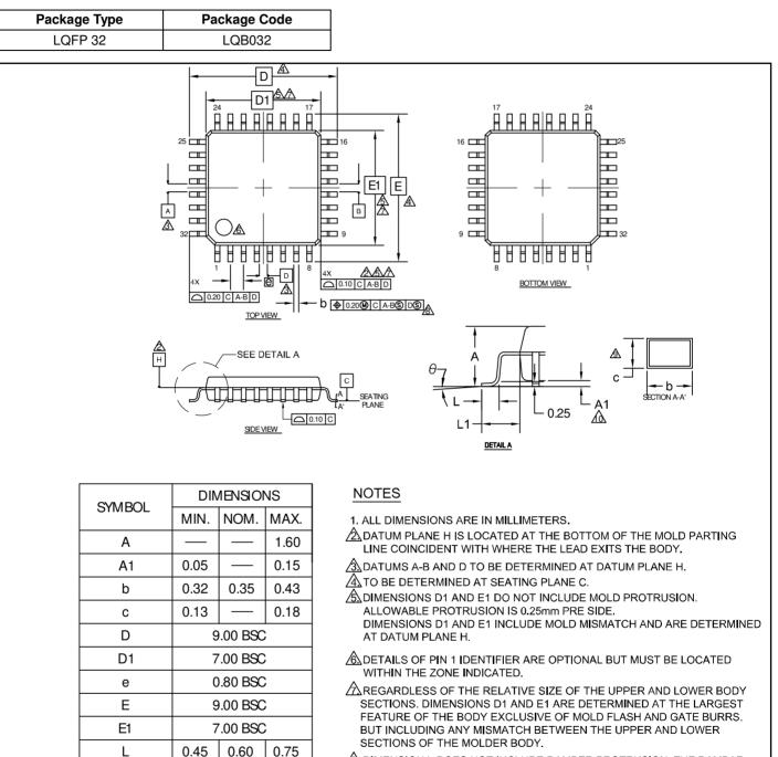
▲ DIMENSION b DOES NOT INCLUDE DAMBER PROTRUSION. THE DAMBAR PROTRUSION (S) SHALL NOT CAUSE THE LEAD WIDTH TO EXCEED b MAXIMUM BY MORE THAN 0.08mm. DAMBAR CANNOT BE LOCATED ON THE LOWER RADIUS OR THE LEAD FOOT.
