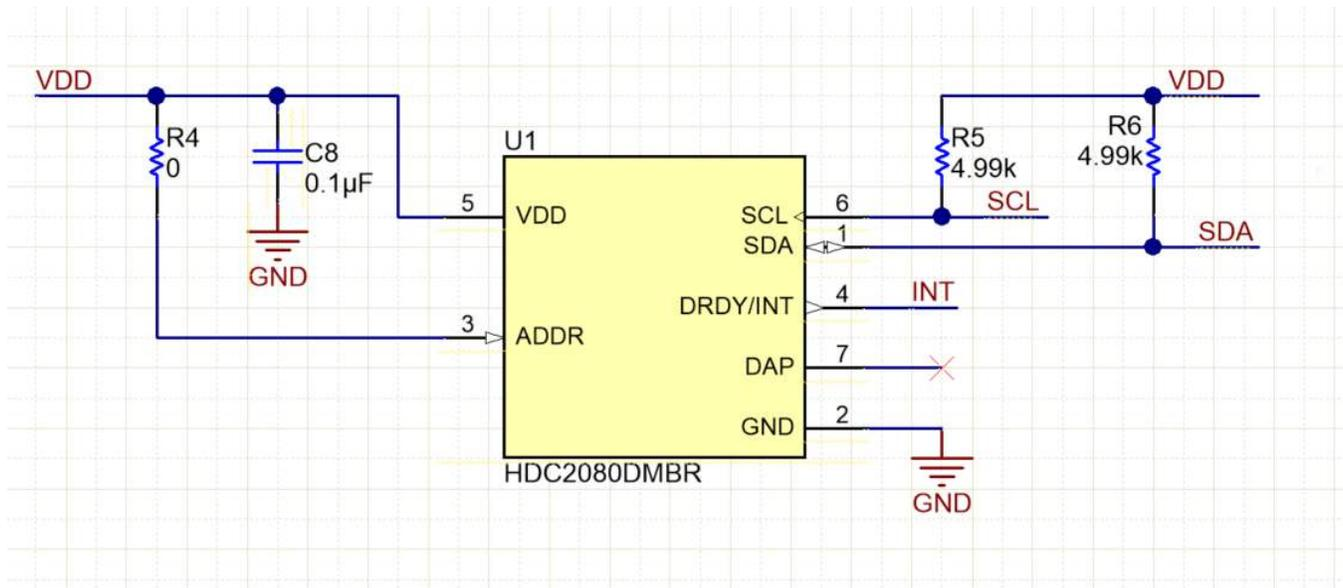
**Figure 2. HDC2080EVM : Sensor Module**
