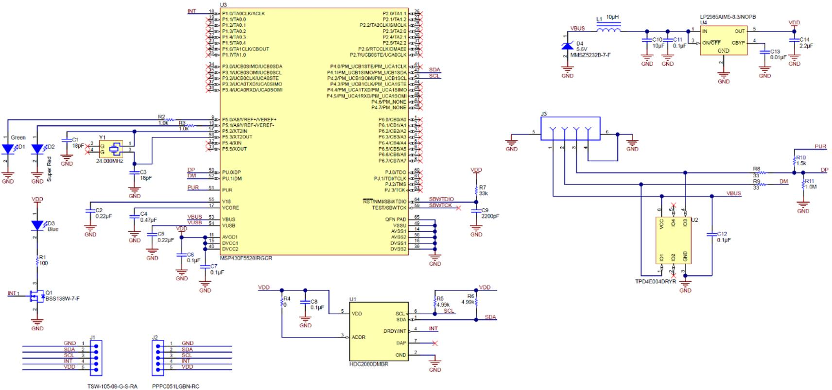
Figure 56. HDC2080EVM Schematic
