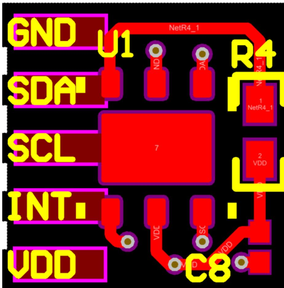
Figure 3. HDC2080EVM: Layout Resistors for I2C Address Setting - Top
