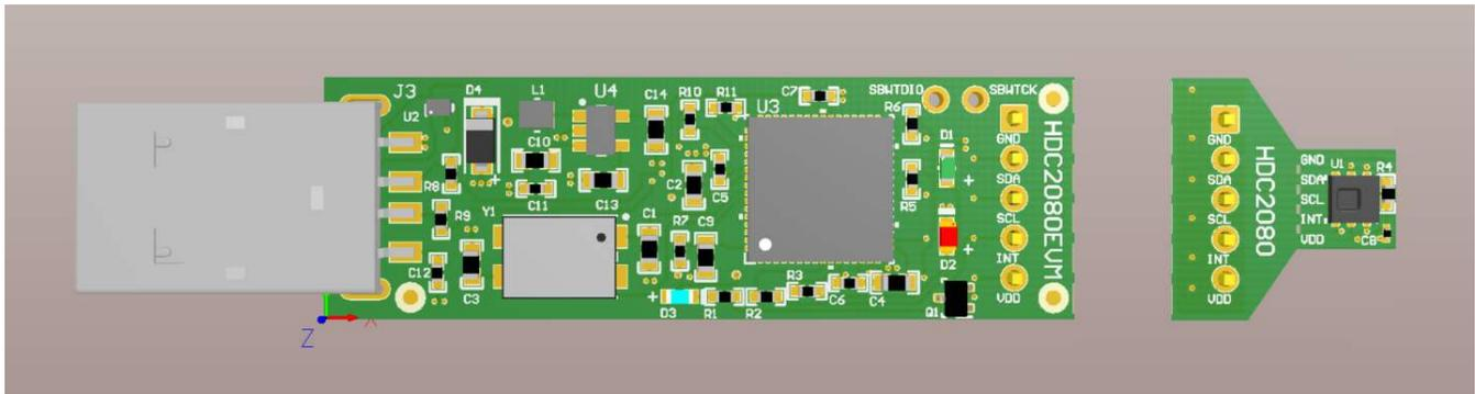
**Figure 12. HDC2080EVM : PC Interface and Sensor Module**
