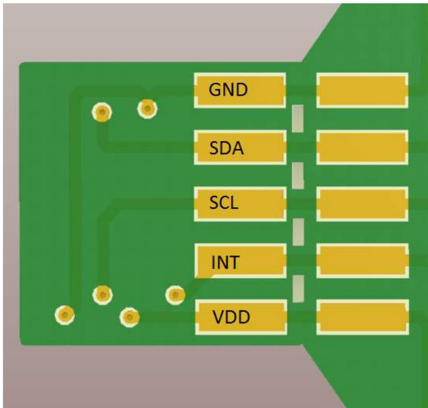
Figure 14. HDC2080EVM : Pads for I2C and Supply of the Smaller Sensor Module
