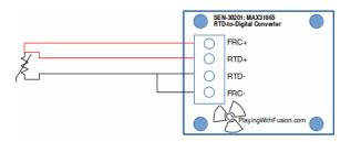
In summary, 4-wire RTDs typically offer the highest accuracy, regardless of distance between RTD and measurement equipment, whereas 2-wire devices may help to reduce system cost.
