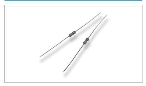
Metal glaze resistors are manufactured using thick film techniques. The ceramic slugs have the thick film applied, the film is fired and end caps are forced onto the slugs, the resistive element is spiralled to value and lead wires are welded onto the end caps. Four layers of coating are applied - the first being a phenolic resin, the other three being epoxy.
