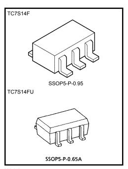
Weight SSOP5-P-0.95: 0.016 g (typ.) SSOP5-P-0.65A: 0.006 g (typ.)
