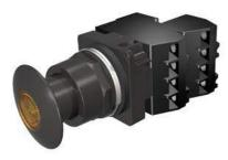
30mm BlackMax, Epoxy Coated Corrosion Resistant Complete Metal Unit Illuminated Push-Pull Operator Transformer type, 120V AC LED Lamp Mushroom Head Cap Small 1 3/4" (44.5 mm) Metal, Black with Amber Lens 3 Position Pull-Momentary/Push-Maintained 1 N.C.+1 N.C. Extra Late Break Heavy Duty Contacts, A600/P600 UL Listed, CSA Certified NEMA 1,3,3R,4,4X,12,13 & Automotive Standards
