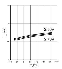
LOW Gain Mode  $\label{eq:supply} \mbox{Supply current vs. Temp. } I_{\mbox{ } CC} = f(T_{\mbox{$A$}}, V_{\mbox{$CC$}})$
