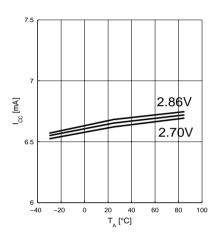
MID Gain Mode Supply current vs. Temp.  $I_{CC} = f(T_{A}, V_{CC})$
