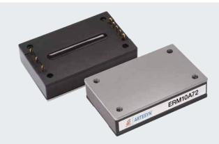
Advanced Energy's Artesyn ERM50 series high performance 50 watt isolated DC-DC converter modules are designed specifically for railway applications. The high input versions feature a 66 to 160 Vdc input that complies with the European EN50155 standard for electronic equipment used on railway rolling stock. There is a choice of four single output models, offering voltages of 5 V, 12 V, 15 V or 24 V.
