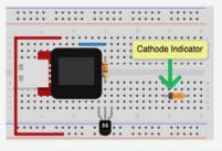
Insert your Diode into points C24 (Cathode) and C28 (Anode).
