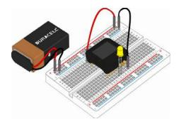
The MicroView is able to detect if the LED is inserted with the correct polarity, if the LED does not blink, remove the LED and turn the pins the other way round and connect them to PIN 4 and PIN 5 of the MicroView.
