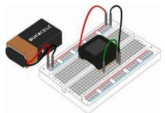
Once you have successfully connected PIN 2 and PIN 8 of the MicroView, a "Well done!" message will be displayed. To proceed to the next simple tutorial, remove the jumper.
