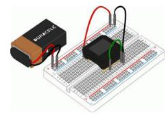
Once you have successfully connected PIN 3 and PIN 8 of the MicroView, a "Well done!" message will be displayed. To proceed to the next simple tutorial, remove the jumper.
