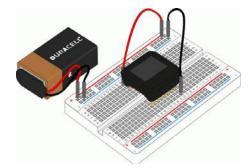
As soon as the battery snap connector is snapped to the 9V battery, the MicroView demo will start.
