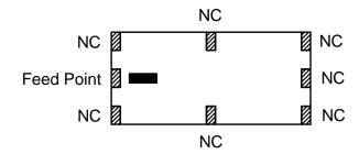
The matching circuit shown has been designed based on the Würth Elektronik evaluation board and cannot be reused. It is recommended to leave a 'Pi' or 'T' type matching circuit space for antenna matching circuit for other boards.
