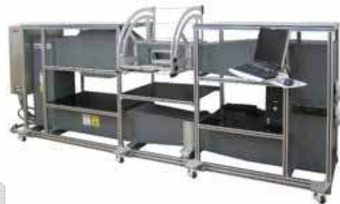
Fig F: FDK Original Wind Tunnel
