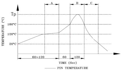
A. Preheating B. Soldering C. Gradual Cooling
