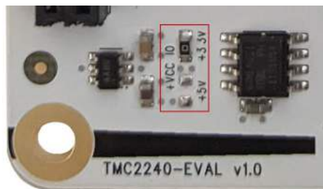
Figure 4: +VCC IO selection near the EEPROM
