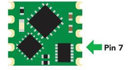
The Interrupt control register adjusts the function of pin 7 (the interrupt output pin).
