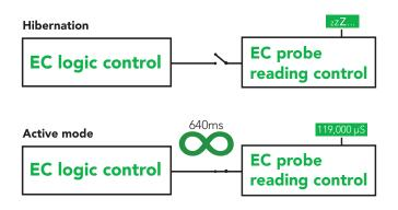
Example code **Activate EC readings** byte i2c\_device\_address=0x64; byte active reg=0x06; Wire.beginTransmission(i2c\_device\_address); Wire.write(active\_reg); Wire.write(0x01); Wire.endTransmission();
