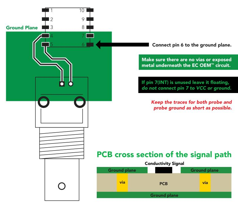
This cross section is an example of how the ground plane protects the Conductivity signal. The ground plane should surround the Conductivity signal, on the top layer as well as the bottom layer.
