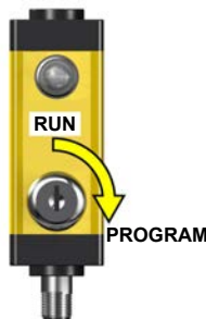
Figure 55. EZA-RBK-1 switch positions and programming status indications
