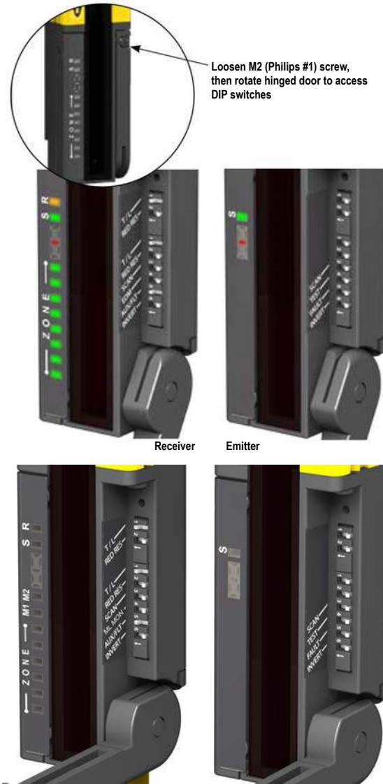
Figure 41. Accessing the configuration switches
