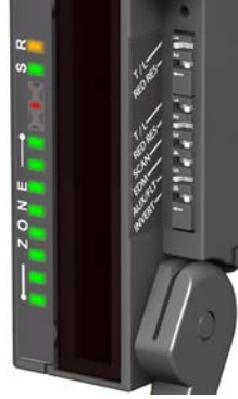
Figure 50. DIP switch configuration to enable cascade installation
