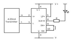
Using an external LED as a high alarm and a switch to acknowledge the alarm (to stop it flashing)
