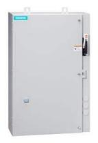
Non-reversing motor starter Size 2 1/2 Three phase full voltage Solid-state overload relay OLRelay amp range 25-100A 190-220/220-240V 50/60HZ coil Combination type 100A circuit breaker Enclosure NEMA type 4/12 Water/dust tight for outdoors Standard width enclosure
