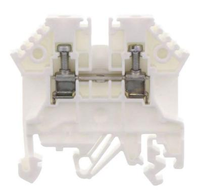
Feed-through terminal, Screw connection, Mounting type:Mounting rail TS 35/7.5 and TS 32, Rated cross-section: 2.5 mm², Width: 5 mm, Colour: White
