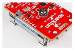
Installing the batteries are easy, but as you install the batteries, make sure you insert the batteries in the same orientation as the silkscreen image between each pair of battery clips. After the batteries are installed, you're all set! You can move the switch on the left side of the board to "ON", and you should see the red power LED come on.
