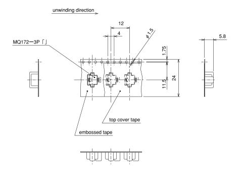
(Note.) The figure above provides the case of a 3 contact type, dimensions shown in such figure are the same as those of a 4 contact type.
