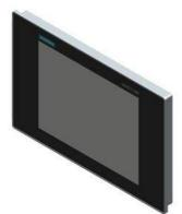
SIMATIC IFP1500 V2 Extended 4:3 15" multi-touch display (4:3) with 1024x768 pixel resolution; built-in unit for 24 V DC; DisplayPort; can be placed up to 100 m away HDBaseT; USB on the rear side; standard Siemens design
