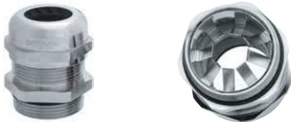
SKINTOP® MS-SC is uniquely designed to address EMI concerns with its simplified grounding feature. In a few easy steps the cable is grounded, strain relieved, and sealed from moisture and dust in accordance with IP68. The cable glands' contact springs establish a continuous electrical path from the shield of the cable to the equipment ground, creating a secure shield connection.
