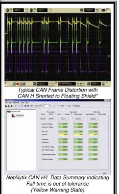
\* Signal captures were obtained using a digital storage oscilloscope on a typical DeviceNet network.
