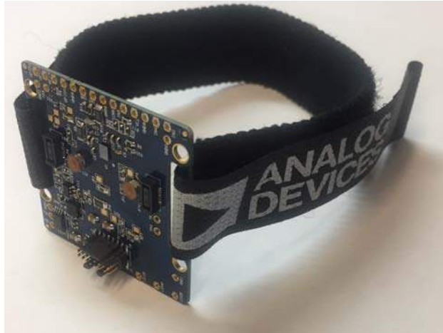
Figure 6. Optional Wrist Strap on EVAL-ADPD4100Z-PPG
