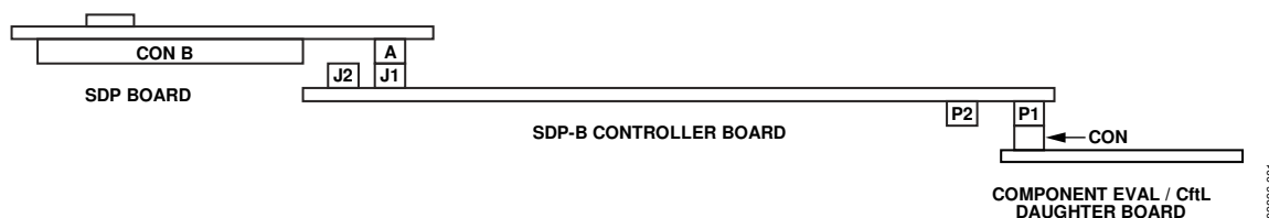
Figure 1. Connecting the SDP Breakout Board
