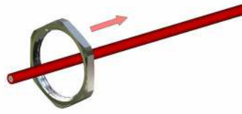
Place counter nut (1) on cable
