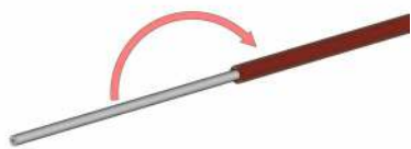
Fold back shield braid over jacket
