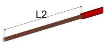
⚠ ONLY when using shielded cable: Remove cable jacket
