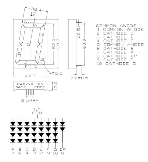
Note: Tolerances unless mentioned  $\pm 0.25$ mm. Unit = mm
