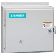
Non-reversing motor starter, Size 1, Three phase full voltage, Solid-state overload relay, OLRelay amp range 3-12a, 240V 50HZ / 277V 60HZ coil, Non-combination type, Enclosure type 12, Dust/drip proof for indoors, Standard width enclosure
