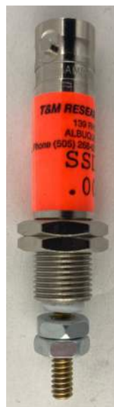
Figure 5. T&M Research SSDN-005 5 m \Omega CVR
