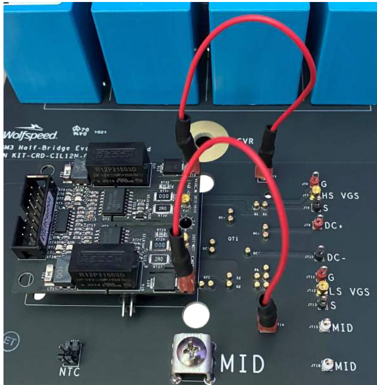
Figure 13. Dual-Channel Gate Driver with DESAT Cable Connections
