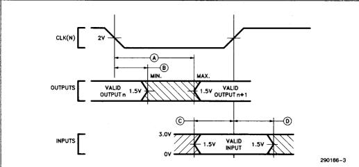
Input waveforms have tr  $\leq$  2.0 ns from 0.8V to 2.0V.
