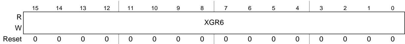
Figure 5-17. XGATE Register 6 (XGR6)
