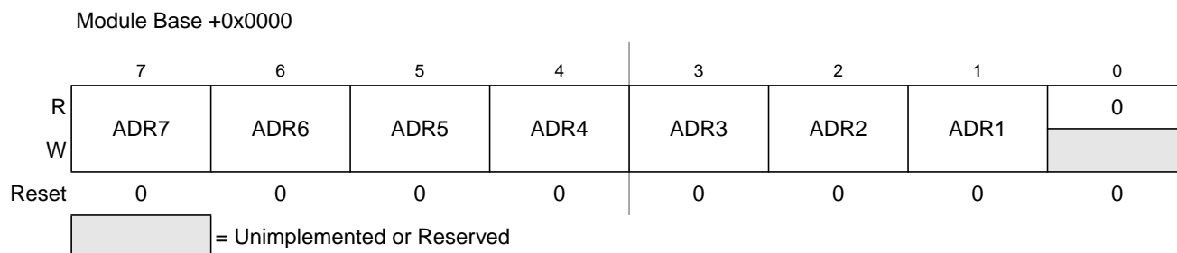
Figure 13-3. IIC Bus Address Register (IBAD)
