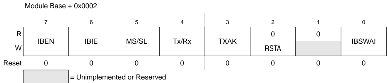
Figure 13-6. IIC Bus Control Register (IBCR)
