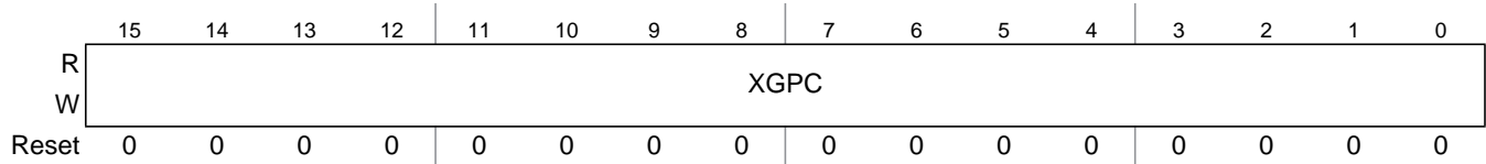
Figure 5-10. XGATE Program Counter Register (XGPC)
