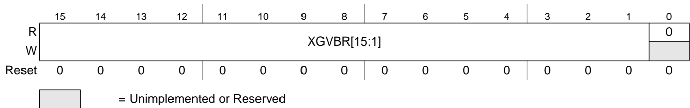
Figure 5-5. XGATE Vector Base Address Register (XGVBR)
