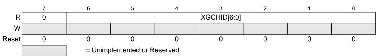
Figure 5-4. XGATE Channel ID Register (XGCHID)
