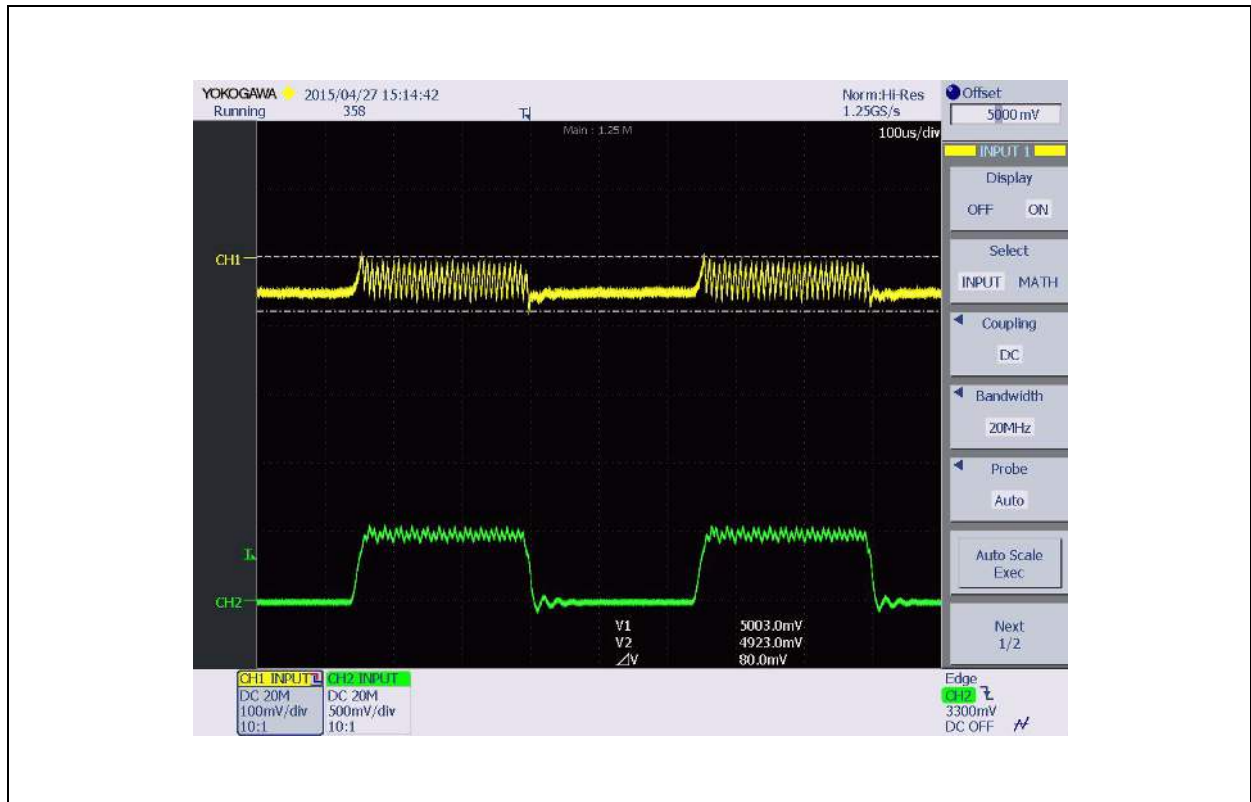
Figure 11: V_{OUT} Behavior When V_{IN} is Stepped Between 3.0V and 3.5V ( I_{LOAD}=100mA , V_{OUT} = 5.0V )
